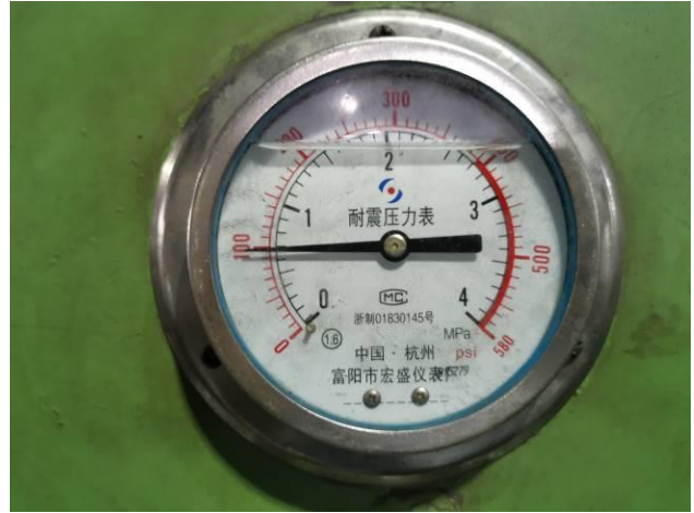
8. Seat test low pressure indicated for Z961Y-63I DN400 Welded Wedged Gate Valve
