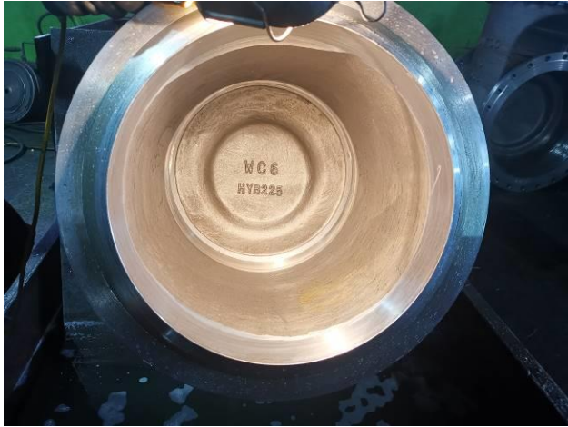
7. Seat without leakage during high pressure test for Z961Y-63I DN400 Welded Wedged Gate Valve-2
