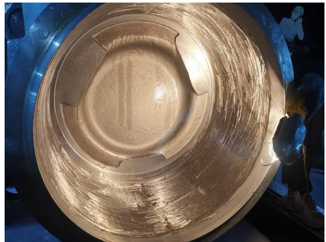
30. Seat without leakage during low pressure test for Z961H-16C DN700 Welded Wedged Gate Valve-2
