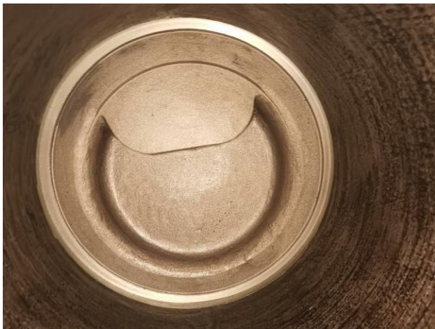
17. Seat without leakage during high pressure test for Z961Y-63I DN500 Welded Wedged Gate Valve-2
