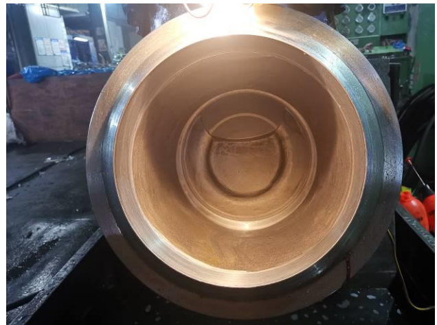
6. Seat without leakage during high pressure test for Z961Y-63I DN400 Welded Wedged Gate Valve-1
