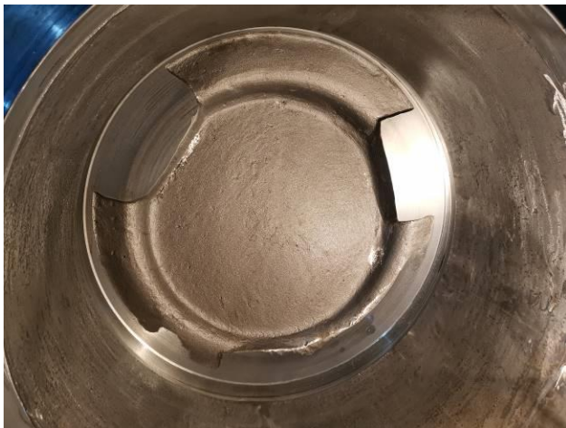
37. Seat without leakage during high pressure test for Z961H-16C DN900 Welded Wedged Gate Valve-2
