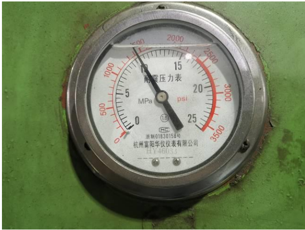
3. Shell test pressure indicated for Z961Y-63I DN400 Welded Wedged Gate Valve
