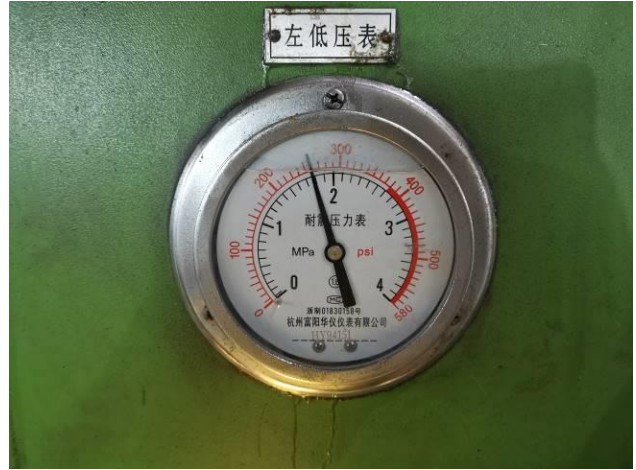
24. Backseat and seat high test pressure indicated for Z961H-16C DN700 Welded Wedged Gate Valve
