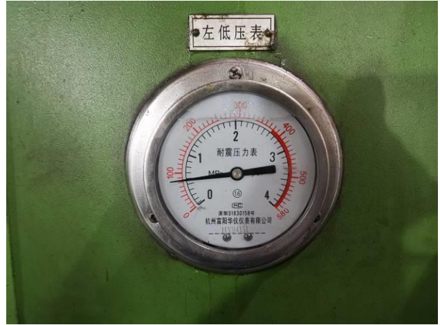
28. Seat test low pressure indicated for Z961H-16C DN700 Welded Wedged Gate Valve
