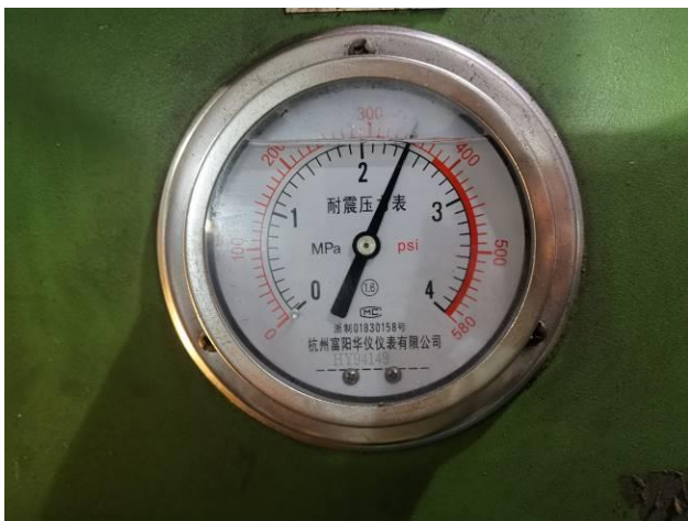
33. Shell test pressure indicated for Z961H-16C DN900 Welded Wedged Gate Valve
