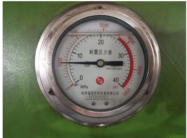
14. Backseat and seat high test pressure indicated for Z961Y-63I DN500 Welded Wedged Gate Valve
