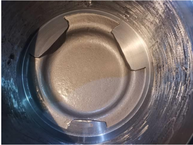
27. Seat without leakage during high pressure test for Z961H-16C DN700 Welded Wedged Gate Valve-2
