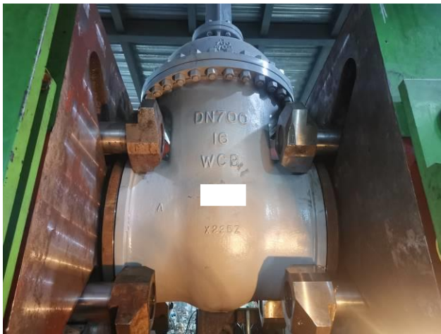
21. Shell pressure test for Z961H-16C DN700 Welded Wedged Gate Valve-1
