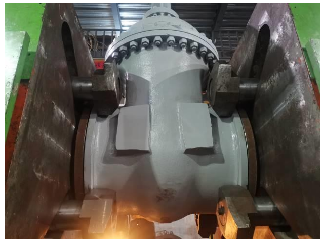
22. Shell pressure test for Z961H-16C DN700 Welded Wedged Gate Valve-2
