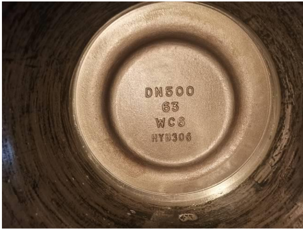
19. Seat without leakage during low pressure test for Z961Y-63I DN500 Welded Wedged Gate Valve-1
