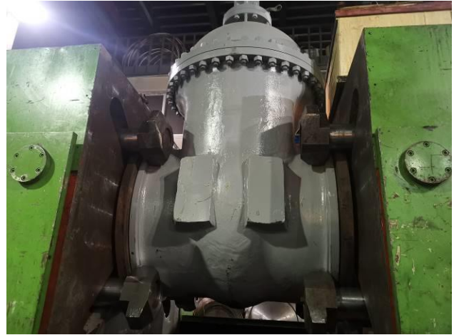
32. Shell pressure test for Z961H-16C DN900 Welded Wedged Gate Valve-2
