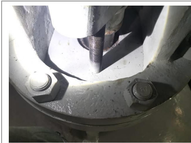
35. Backseat without leakage during high pressure test for Z961H-16C DN900 Welded Wedged Gate Valve
