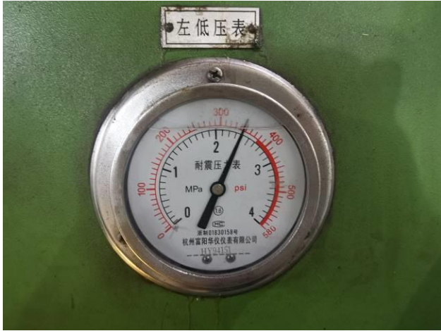
23. Shell test pressure indicated for Z961H-16C DN700 Welded Wedged Gate Valve
