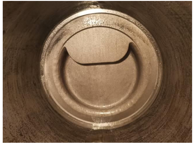
20. Seat without leakage during low pressure test for Z961Y-63I DN500 Welded Wedged Gate Valve-2
