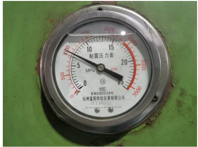
4. Backseat and seat high test pressure indicated for Z961Y-63I DN400 Welded Wedged Gate Valve
