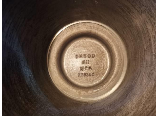
16. Seat without leakage during high pressure test for Z961Y-63I DN500 Welded Wedged Gate Valve-1
