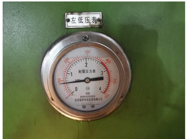
18. Seat test low pressure indicated for Z961Y-63I DN500 Welded Wedged Gate Valve
