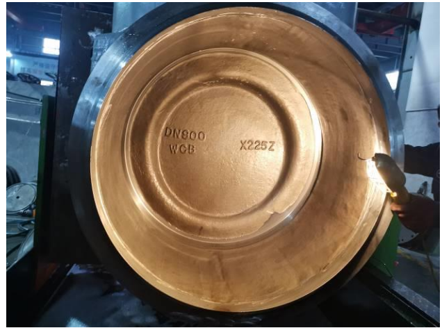
36. Seat without leakage during high pressure test for Z961H-16C DN900 Welded Wedged Gate Valve-1
