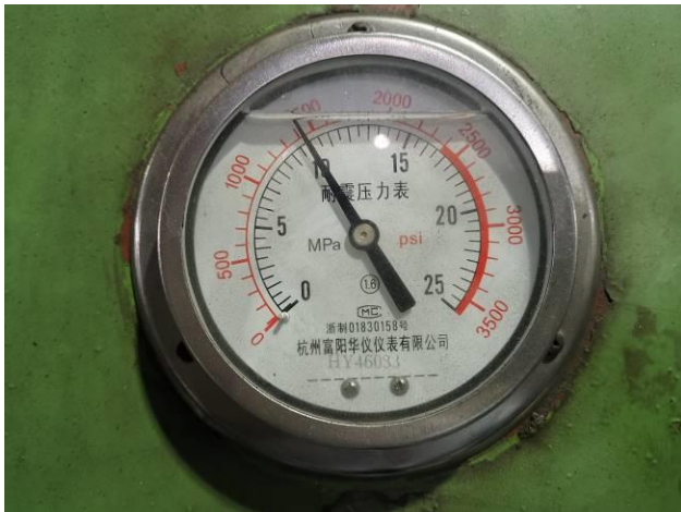
13. Shell test pressure indicated for Z961Y-63I DN500 Welded Wedged Gate Valve
