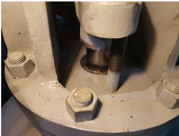
25. Backseat without leakage during high pressure test for Z961H-16C DN700 Welded Wedged Gate Valve
