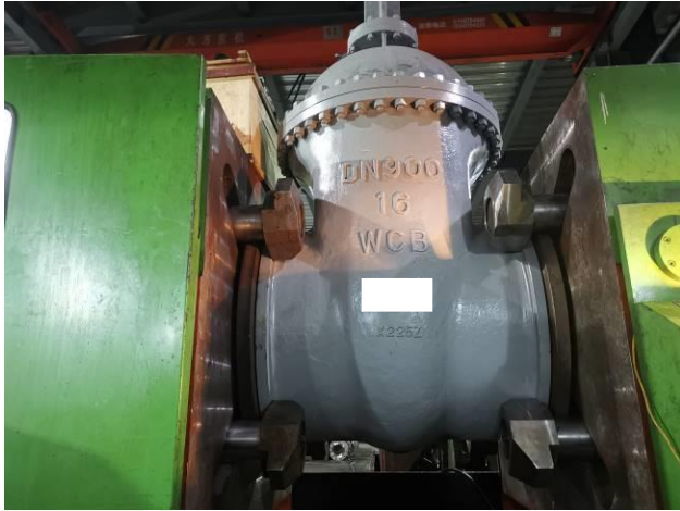
31. Shell pressure test for Z961H-16C DN900 Welded Wedged Gate Valve-1
