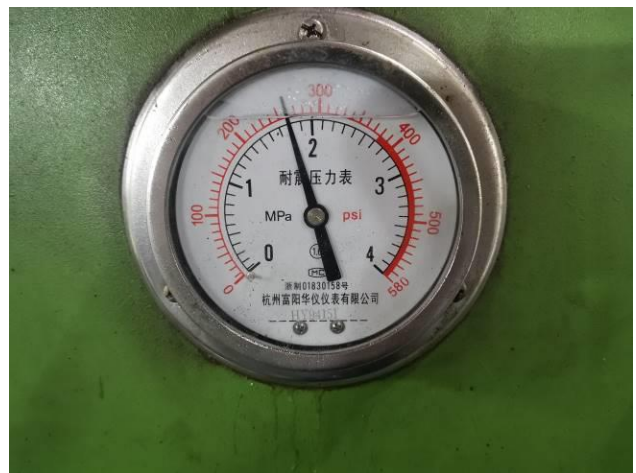
34. Backseat and seat high test pressure indicated for Z961H-16C DN900 Welded Wedged Gate Valve
