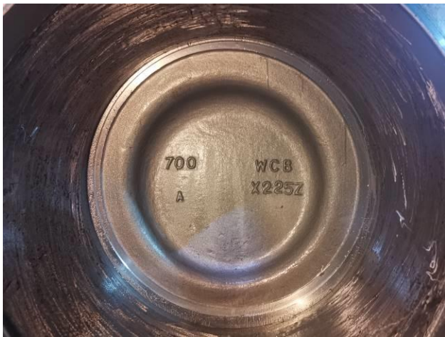
29. Seat without leakage during low pressure test for Z961H-16C DN700 Welded Wedged Gate Valve-1
