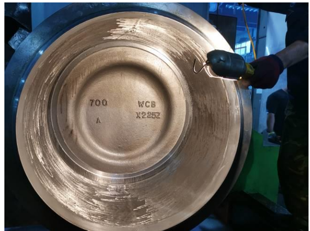
26. Seat without leakage during high pressure test for Z961H-16C DN700 Welded Wedged Gate Valve-1
