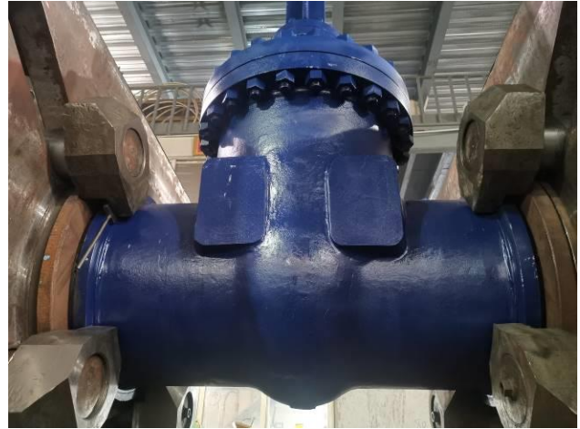
12. Shell pressure test for Z961Y-63I DN500 Welded Wedged Gate Valve-2
